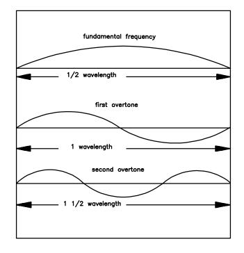
Fig. 11. A vibrating violin string showing the fundamental frequency and the first and second overtones
